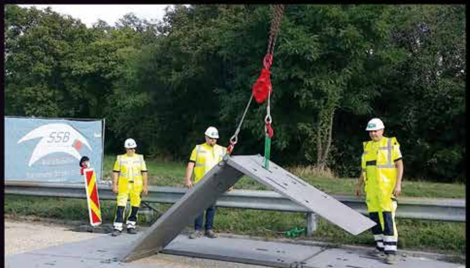
Scrutinising eyes during a function test of an MMBS element.
