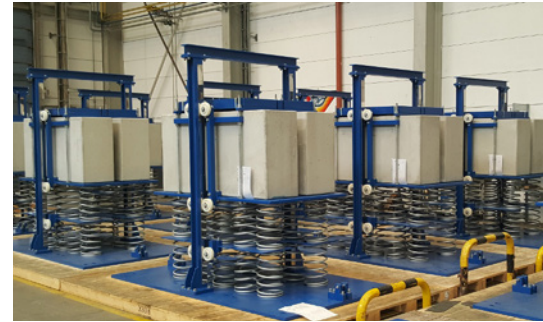
The Spring-Mass-Damper in the MAURER production hall.
