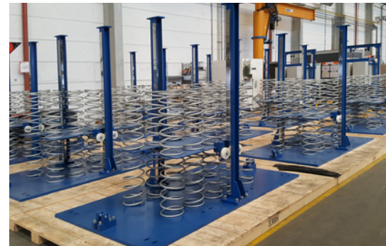
Springs for Mumbai: They are made of extremely hardened spring steel so that they can permanently withstand the high vibration amplitudes of \pm 400 mm. The vertical guides with ball-bearing rollers, which keep the mass "on track", are clearly visible at the front.
