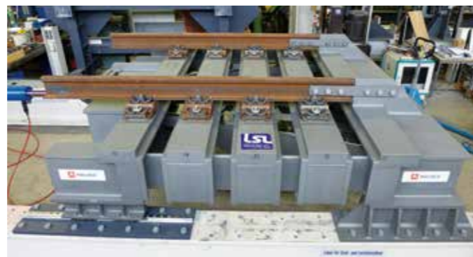
MAURER Guided Cross Tie load test in test lab of Prof. Bucak, Augsburg / Germany
