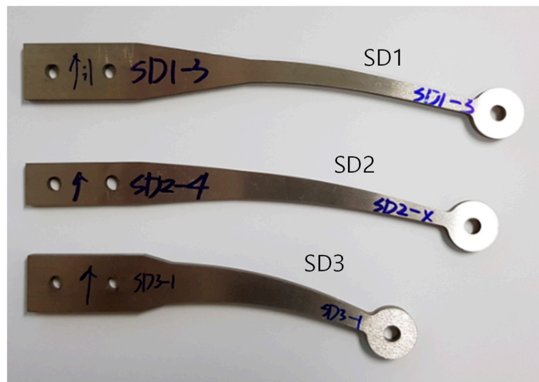
Figure 17. Deformed shapes of steel dampers after the maximum displacement loads.
