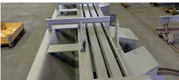
Expansion joint with Fuse Box
