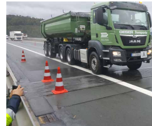
Roll over test MSM® Swivel Joist Expansion Joint
